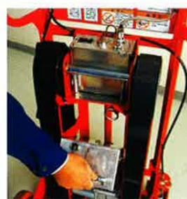
▲Battery pack can be changed with one-touch operation
